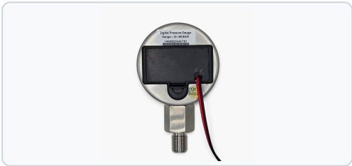
Close the cover through the prepared cable notch; do not pinch the cable.
